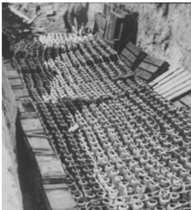
Fig. 2-42. Dumping weapons into the sea was not the Allies' only method of disposing of them. These 150-mm German nitrogen mustard (HN-3) rockets are wired with prima cord for destruction. Photograph: Chemical and Biological Defense Command Historical Research and Response Team, Aberdeen Proving Ground, Md.
