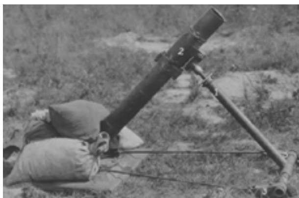
Fig. 2-17. An experimental 4.2-in. chemical mortar, showing (1) the standard, (2) the barrel with the shock-absorbing mechanism, and (3) the tie rods connecting the standard to the baseplate. This weapon differed from the Stokes mortar, its predecessor, in that it was easier to set up and it was rifled; the spiral grooves can be seen on the inside of the barrel at its muzzle. Photograph: Chemical and Biological Defense Command Historical Research and Response Team, Aberdeen Proving Ground, Md.
