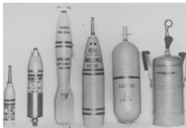
Fig. 2-18. The chemical weapons of the 1920s and 1930s. From left to right: the 75-mm mustard shell; the 4.2-in. white phosphorus shell; the M1 30-lb mustard bomb; the Mk II 155-mm mustard shell; the Livens phosgene projectile; and the Mk I portable chemical cylinder. Photograph: Chemical and Biological Defense Command Historical Research and Response Team, Aberdeen Proving Ground, Md.
