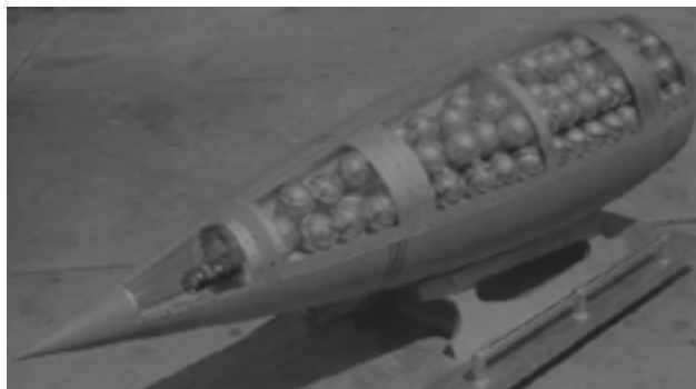
Fig. 2-53. A chemical warhead for the Honest John rocket. It was designed to break apart and disperse the spherical bomblets of nerve agent. Photograph: Chemical and Biological Defense Command Historical Research and Response Team, Aberdeen Proving Ground, Md.
