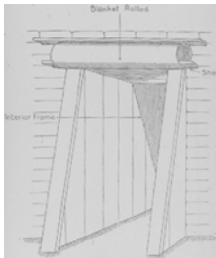
Fig. 2-12. Early attempts at collective protection during World War I included the dugout blanket, which was used to cover the doorways to dugouts. Reprinted from Army War College. Methods of Defense Against Gas Attacks . Vol 2. In: Gas Warfare . Washington, DC: War Department; 1918: Figure 18.
